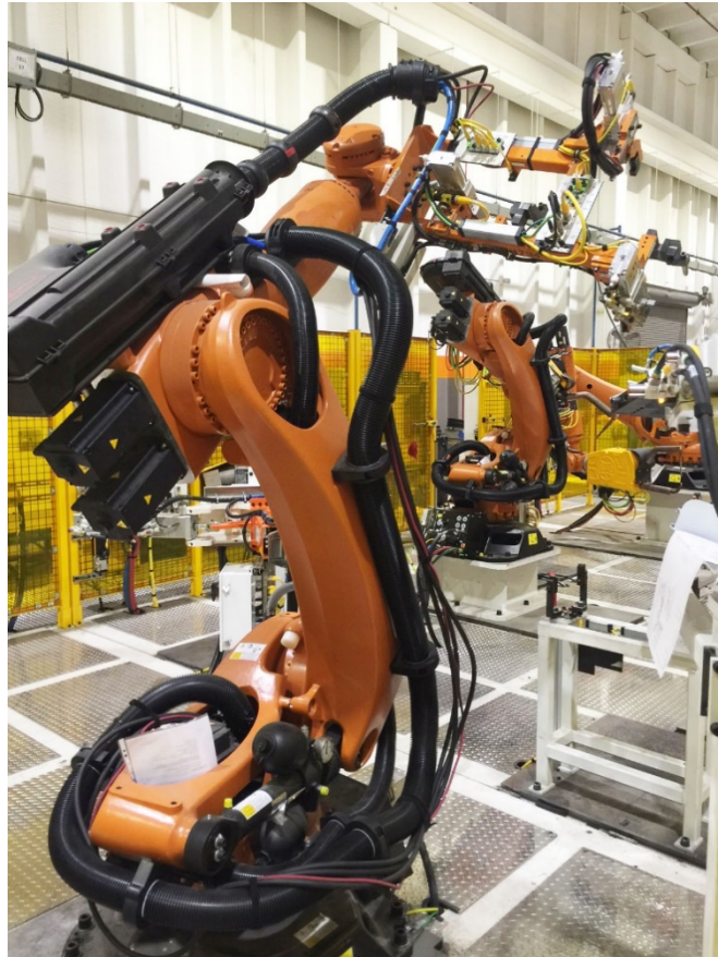
Figure 11: Example of cable management solution.
